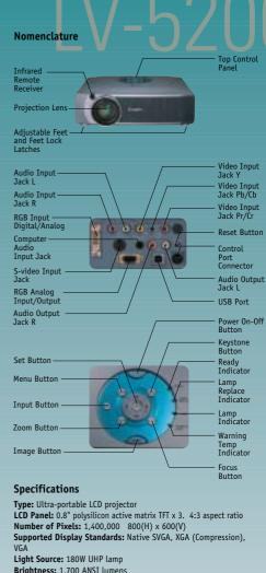
Light Source: 180W UHP lamp Brightness: 1,700 ANSI lumens Uniformity: 85% (corner to center) Contrast Ratio: 400:1
