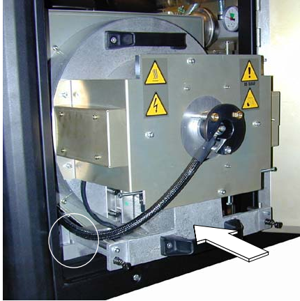
Image 7-4 Securing the lamp unit
