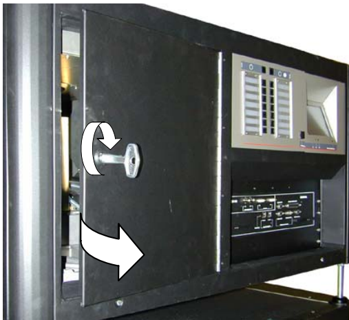
Image 7-1 Access to lamp casing
