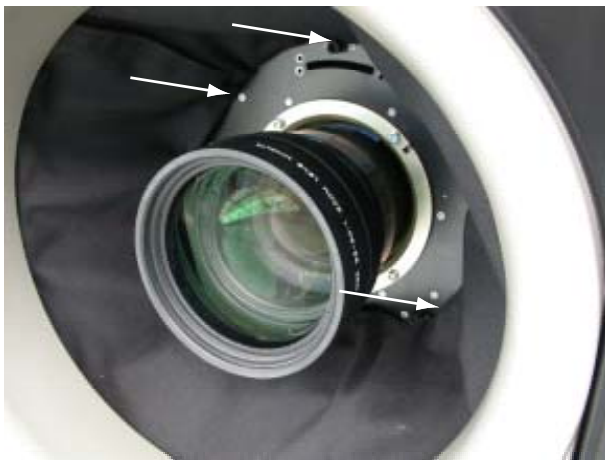
Image 9-4 Dust sock removal
