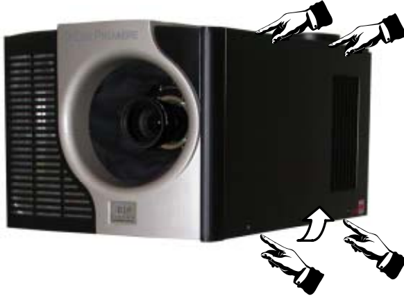
Image 9-3 Right side cover removal
