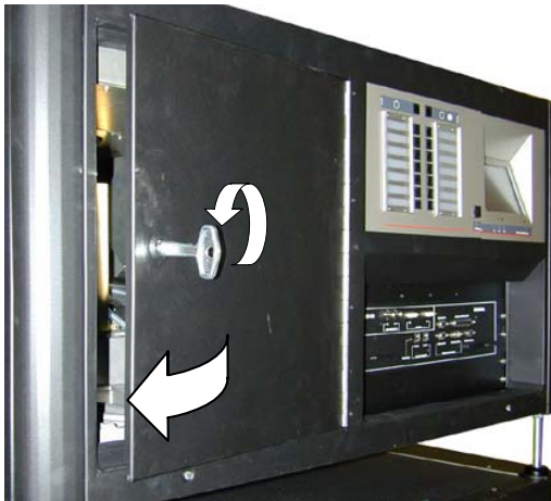
Image 7-5 Locking the lamp house door
