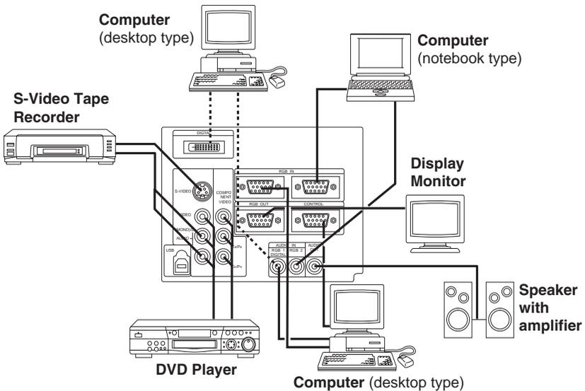
**NOTE** • When connecting with a notebook computer, set the proper RGB external image output (setting CRT display or simultaneous display of LCD and CRT). Please read instruction manual of the notebook for more information.
